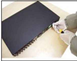
① disassemble the screw
