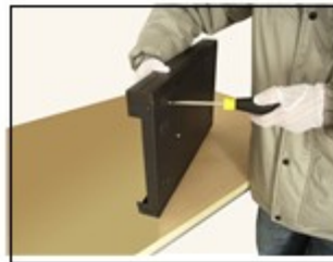
④ fix the screw of hard disk
