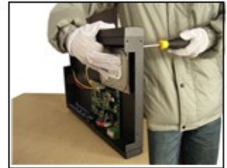
③ fix the screw of hard disk
